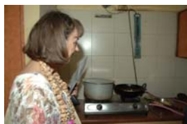
26 th April 2009, Sulabh's campus: Cooking with gas received from the composting of the human excreta from the nearby public toilet.
